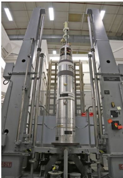
One of the ACES payloads on the spin–balance table at Wallops. Credit: NASA Photo/Berit Bland
